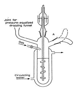
side tube "A" of the apparatus. The reaction mixture quickly became black, and a seemingly homogeneous system was formed. Gas absorption set in, the volume of which was measured with a gas burette. Experiments usually lasted 1–6 h, during which time the rate of gas absorption gradually diminished.
